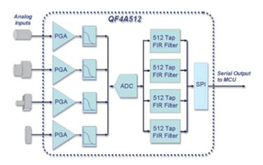
from Quickfilter Technologies at www.quickfiltertech.com). So, with the development kit, we have four programmable amplifiers, low pass filtered for anti-aliasing, a fast 16-bit A/D converter, and four software programmable FIR filters, all connected to a USB port.
